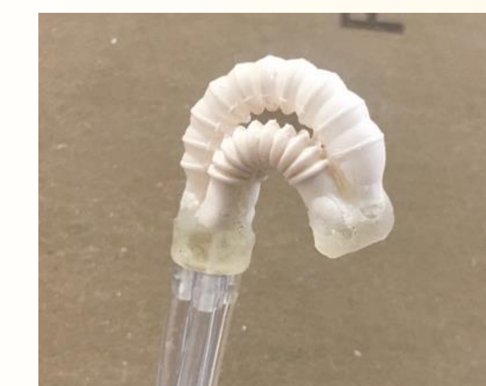
Figure 8: New bellow end-effector approaching retroflexion configuration
