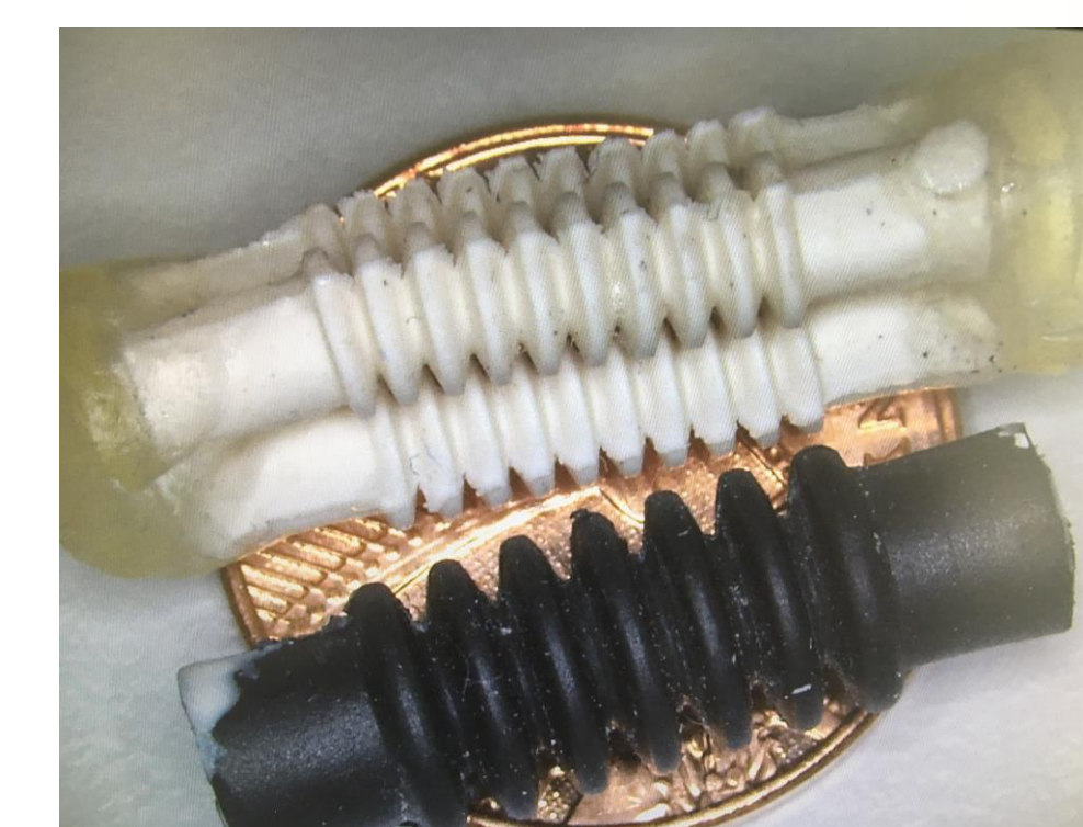
Figure 7: Three new bellows next to current bellow superimposed on British penny
