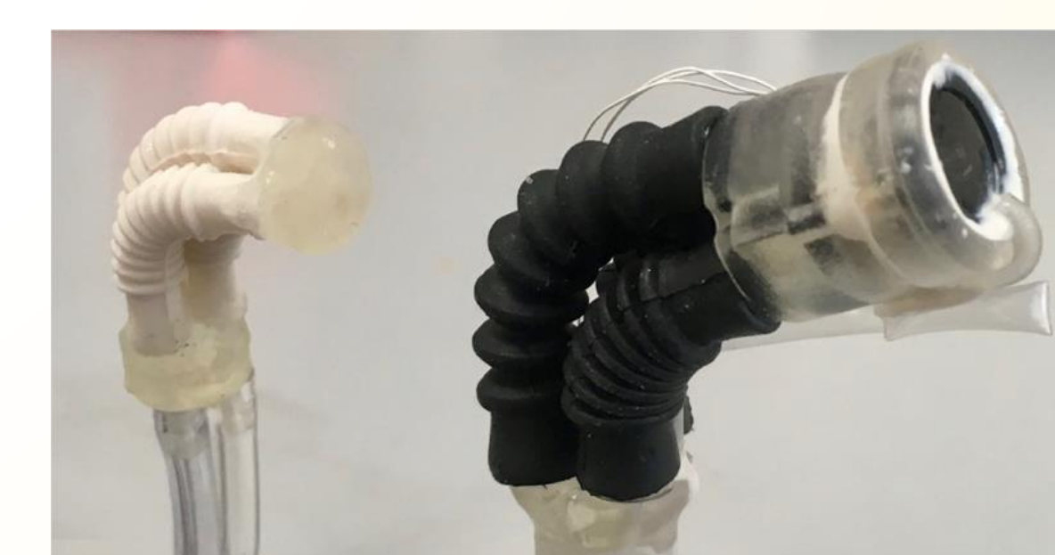
Figure 9: New end-effector tip compared to current tip
