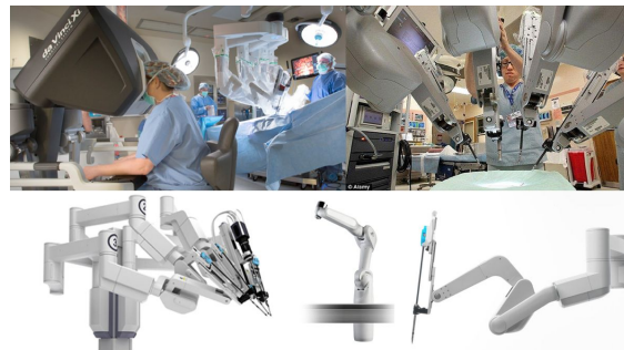
Figure 1: Intuitive Surgical's DaVinci Surgical System® Utilizes a Four Arm System Controlled by a Medical Doctor to Perform Operation
